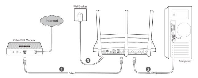
Figure 2-1 Hardware Installation
